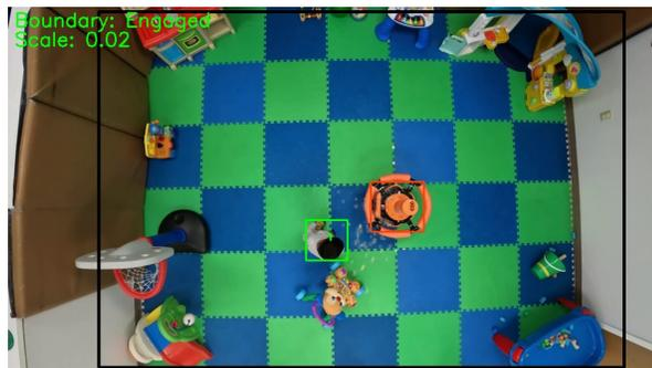
Fig. 3. A frame from OverTrack use during post hoc data extraction. The thick black rectangle surrounding the play space denotes the play space boundary, the orange bounding box marks the robot, and the green bounding box marks the participant. The text in the top left corner indicates that the boundary is set and shows the scale in use for distance measurements.
